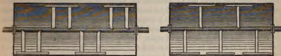
FIGS. 9a AND 9b.—ARRANGEMENT OF MASTIC MIXER.
